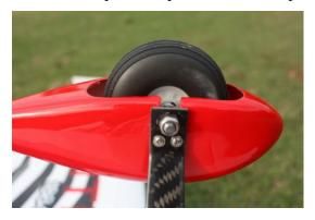
2.4 Bolt the main gear to the bottom of the fuselage using the supplied bolts
