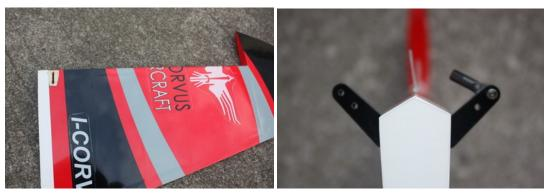
4.3 Connect CA hinges for rudder.
