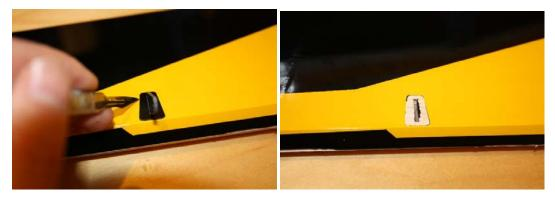
1.3 Use some fine sandpaper to roughen up the root of control horn where will be glued into the slot.
