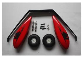
2.2 Install the wheel axles to the landing gear and tighten the nylon-insert lock nut. Install one wheel collar onto the axle. Use a second wheel collar as a guide to leave a gap on the inboard of the axle. Use a small drop of thread-lock and tighten in place. Slide the wheel onto the axle and install a second wheel collar also using thread-lock on the set screw.
