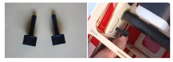
10.3 Side force generators Assembly, cut the wing film needed to be instal the SFG. Fixed the SFG Use M3X12 Hexagon socket screw and washers.
