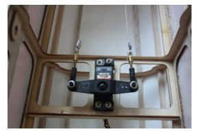
4.7 Check the operation of the rudder using your radio and make sure there is no binding and the cables are adjusted properly. You may have to tighten the cables after a few flights as they may stretch slightly from the initial installation.
