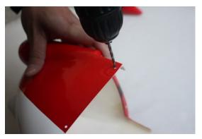
7.4 Secure the cowl with 3X12mm self-threading screws.
