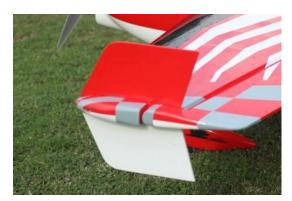
10.5 Check all control surfaces for secure hinges by performed a slight tug on the control surfaces and observing if there is any give in the hinges. Check all control rods, ball links, servo screws, etc. for proper operation and installation.
