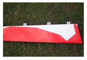
1.6 Cut the covering from the aileron servo slots from corner to corner and iron down inside the openings. Connect servo wire extensions to your servos and secure the connections with the supplied clips. Feed the servo wires into the wing and out the root. The screw holes for servo mounting are laser pre-drilled, it is advisable to apply some thin CA to strengthen them, Install the servos and screw firmly in place.
