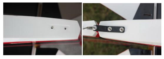
5.4 Drill a hole on the bottom of rudder, 70-100mm away for the hinge line. Secure the tail wheel spring with provided self-threading screw.
