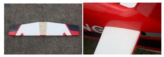
3.4 There is an option to use one servo or two servos for the elevator. If using one servo, the twohalves of the elevator need to be connected by the included fiberglass bar with glue as shown below. The picture is for illustration only. Actually, the connection of the 2 parts needs to be performed before the hinges are connected.
