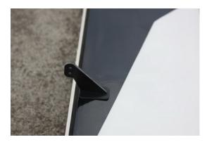
1.5 The slots for CA hinges are pre-cut. Insert CA hinges half way into the hinge slots on aileron, apply a drop of thin CA to secure the hinges. Then insert all hinges into slots on the wing at once, align aileron with the wing, move the aileron up and down a few times to reach the minimal hinge gap while still allowing full deflection of the aileron. When satisfied, apply more think CA on both top and bottom sides of each hinges.
