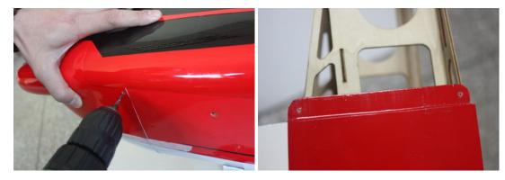
7.3 Enlarge the holes on cowl with 3mm drill bit.
