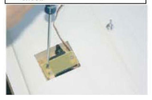
Drill 4mm hole in aileron and install the control horn and linkage.
