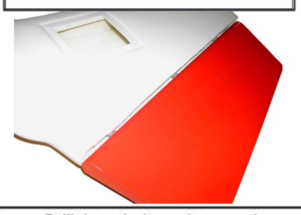
24. Drill 4mm hole and epoxy the alloy connector.
