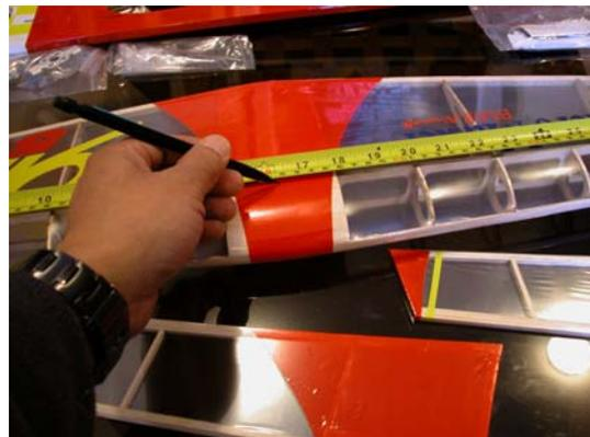
4. Insert the wing into the wing slot. Make sure both side of the wing is the same length. Draw lines along both side of the fuselage.
