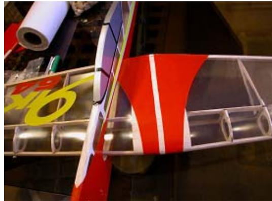
**Peer off the covering where been cut. Put it back into the fuselage wing slot,**
