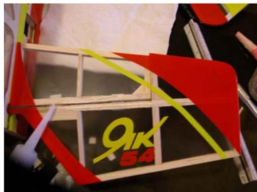
**6. The next step is to CA the elevator. This step has to be done before you CA the vertical fin.**
