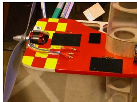
**14. As the photo shown to the right, is a 910 mah 3 cell Li-po pack. The motor is a 370 size 960 KV out-runner and a 20A controller.**
