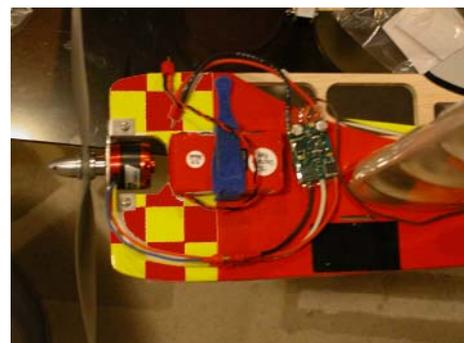
**15. Now hook up the battery and the controller, turn on your radio. Then start make up the push rods for every control surface.**
