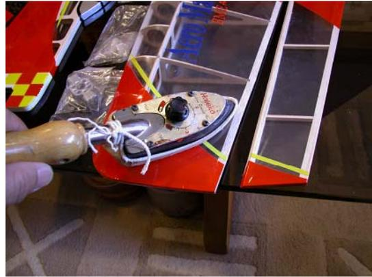
2. After the ironing job. You can start the assembling by cutting out the covering where they should be open, such as servo mount, wing slot etc.
