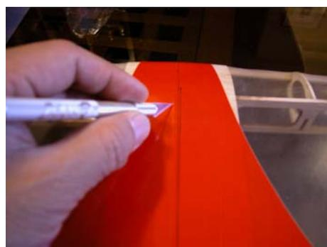
Then cut off the covering where the CA is going to apply to.
