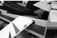
It is important that care is taken when aligning the rear stab. Measure each side to make sure that an equal amount shows on each side.
