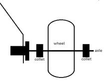
Do not tighten up the collets yet as the wheel needs to be fitted an equal distance within the wheel pant.
