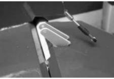
• The area on the horns that goes inside the elevator needs to be roughed up with sandpaper. This allows a better glue joint.
