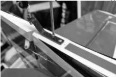
• Drill a hole in the base of the rudder for the rudder steering guide.
