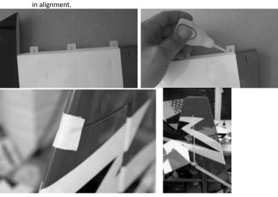
• Glue the rudder horns through the rudder with CA. Use the ball joint and bolt while gluing to maintain alignment.
