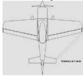
• Glueing – Once you think you are ready to glue, measure again. We recommend 2 methods for gluing. Either remove the covering on the area that is covered by the fuselage and glue with epoxy or leave the covering on and glue with thin cyno. Wicking in thin first, if a large gap is visible then use medium or thick. Remember to wick in small amounts at a time keeping the plane level, this will ensure the glue stays where it needs to be
