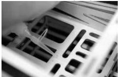
• Using servo screws fix the servo in place, note the spline is towards the front of the plane
