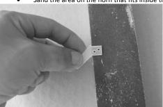
• Glue the rudder hinges into both the rudder and fin using CA glue. Remember to use vaseline on the hinge joint. While drying use tape to keep it in alignment
